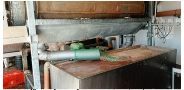
Raw effluent from a factory poultry slaughtering area before being directed to effluent treatment system
